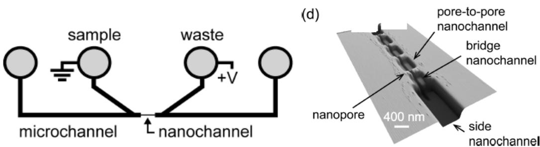
Left - Schematic of an in-plane glass nanofluidic device with two V-shaped microchannels separated by a nanochannel with four pores in series.<sup>6</sup> Right – Atomic force microscope (AFM) image of a 4-pore nanofluidic device.<sup>6</sup>
